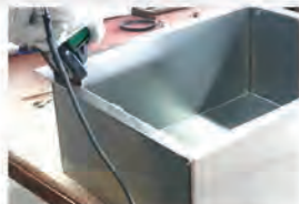
Grinding & Buffing: a grinding machine is used to grind and buff the sink to ensure an even surface and a fine, brushed finish.
